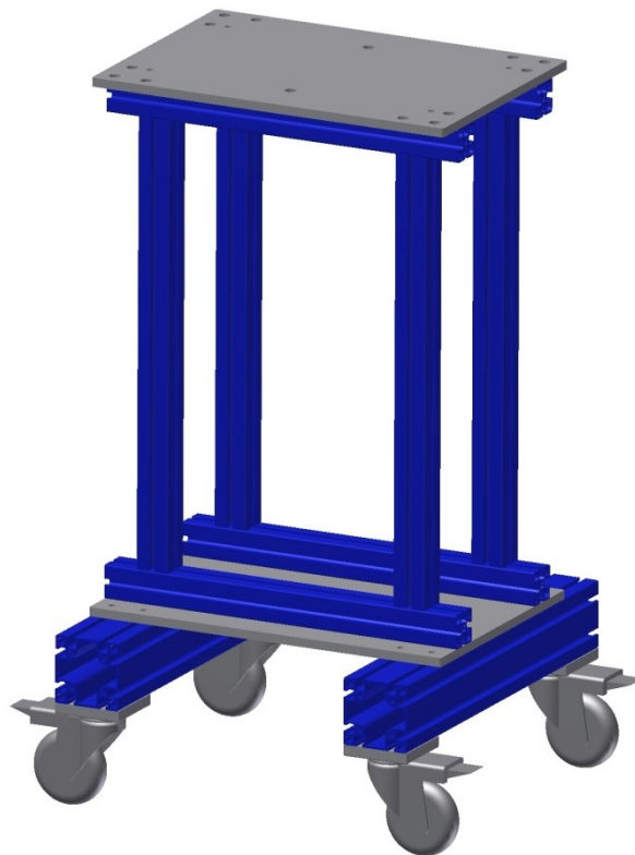
Figure 28: Support stand, 2 required
